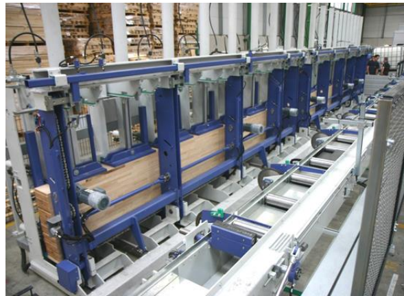
Pressing force is applied from above via pressing shoes
